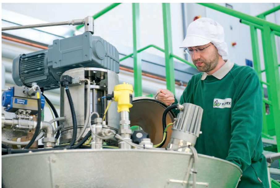
Extract preparation - vacuum distillation system
